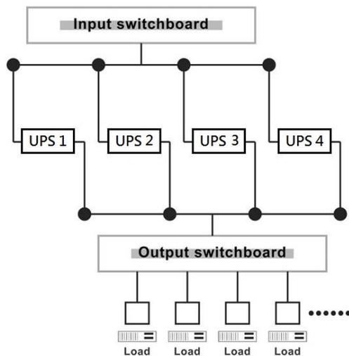
9) Do not switch on the output breaker of each UPS, switch on the input breaker of the each UPS, the UPS should work in bypass with output, observe their display to check if there are any warning or fault information, measure the output voltage of each UPS separately to check if the voltage difference between them is less than 1V. If the difference is more than 1V, check the wiring.
