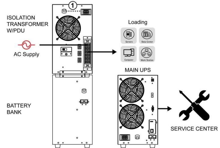
Step 3: When UPS is returned from repair service, please connect cable ①, cable ②, cable ③ of step 1. Make sure all cables are firmly connected.
