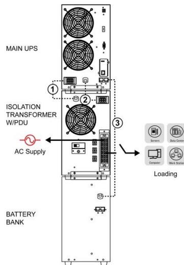
Step 2: Main UPS box can be sent to repair service. During UPS maintenance, you can connect UPS AC input connection cable to UPS AC output connector, refer to below cable ①. Turn on input breaker of mains to supply power to loadings.
