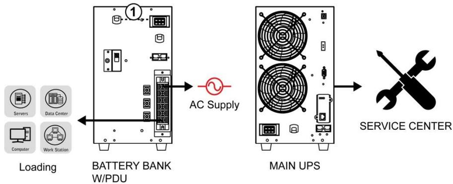
Step 3: When UPS is returned from repair service, please connect cable ①, cable ②, cable ③ of step 1. Make sure all cables are firmly connected.
