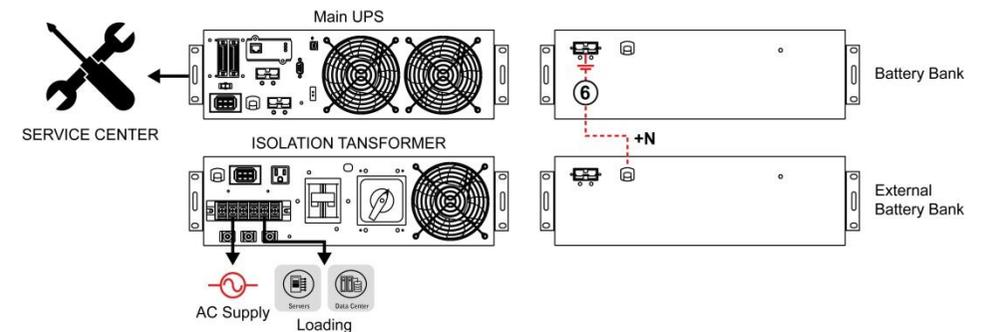
Step 3: When UPS is returned from repair service, please connect cable ①, cable ②, cable ③, cable ④, cable ⑤ of step 1. Make sure all cables are firmly connected, and then turn on the input breaker of mains and change over the maintenance bypass switch from “MAINT.” to “INV.”, lastly , lastly press “ON” button to turn on the UPS.
