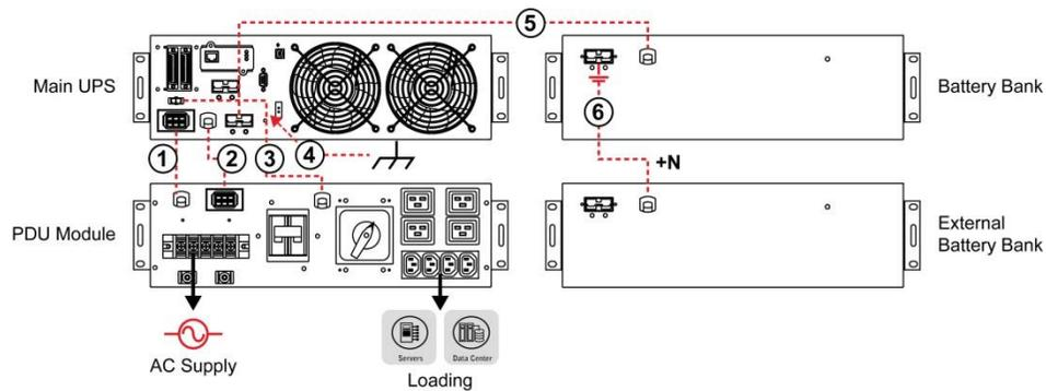
Step 2: Main UPS box can be sent to repair service. The load connected on PDU module will continuously be supplied by AC mains.
