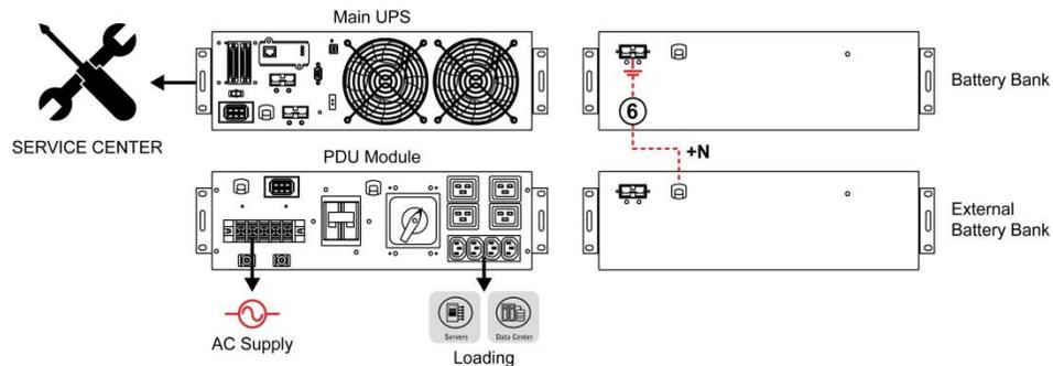
Step 3: When UPS is returned from repair service, please connect cable ①, cable ②, cable ③, cable ④, cable ⑤ of step 1. Make sure all cables are firmly connected, and then turn on the input breaker of mains and change over the maintenance bypass switch from “MAINT.” to “INV.”, lastly press “ON” button to turn on the UPS.
