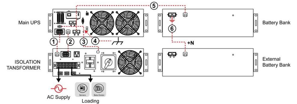
Step 2: Main UPS box can be sent to repair service. The load connected on Isolation Transformer box will continuously be supplied by AC mains.
